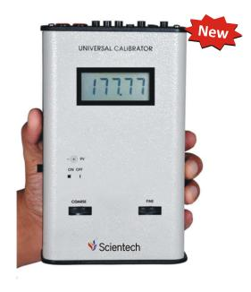
**Scientech 2435T Universal Calibrator** is a micro-controller based precision instrument designed for sourcing and measuring Ohm, RTDs, mA, mV, T/Cs and V signals. It is designed to calibrate a broad spectrum of instruments and retain its precision and repeatability over long periods in severe environmental conditions. An exceptionally stable voltage/current source provides continuously variable precision output signals with two ten-turn potentiometers.
