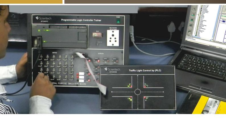
**Traffic Light Control Scientech 2423A** enables Students and practicing Engineers to gain invaluable practical experience of the principles and application of Programmable Logic Controllers.
