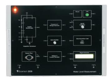
**Scientech 2309 Water Level Measurement** is designed to learn concept of Water Level Measurement. It helps students & industry professionals to understand operation of level sensors in detail. Built-in On/Off Controller is also provided with audio & visual indicators. It also has a PC interface through USB for more interactive understanding of Water Level Measurement. User can also take a direct printout if desired.
