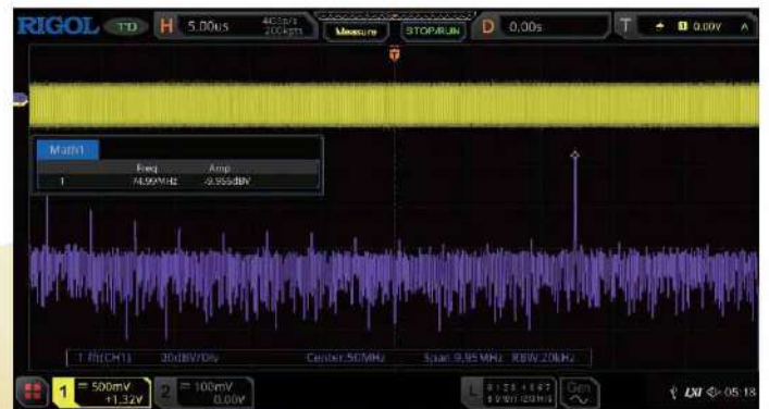
With the near–field probe, you can easily observe the spectrum peak in the frequency domain when the probe approaches to the radiation leakage point.
