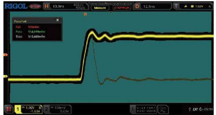
The Pass/Fail test function can quickly make a statistics on the occurrence probability of the signal exceptions.
