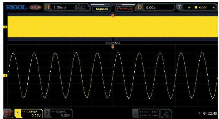
With up to 100 M memory depth, you can capture 12.5 ms of waveforms while maintaining a sample rate of 4 G, without causing the waveforms to be distorted.
