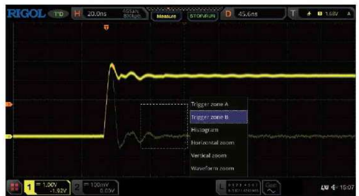
Draw a rectangle on the transient exception signal and select Trigger zone A.
