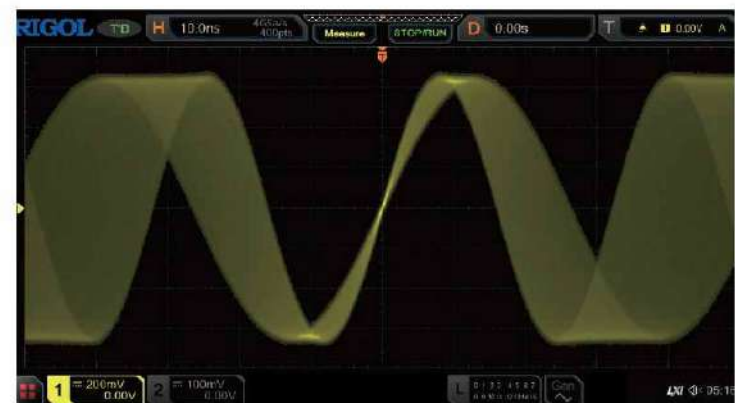
Changes of each frame of waveforms of the sweep signal can be clearly observed in the highly refresh mode.
