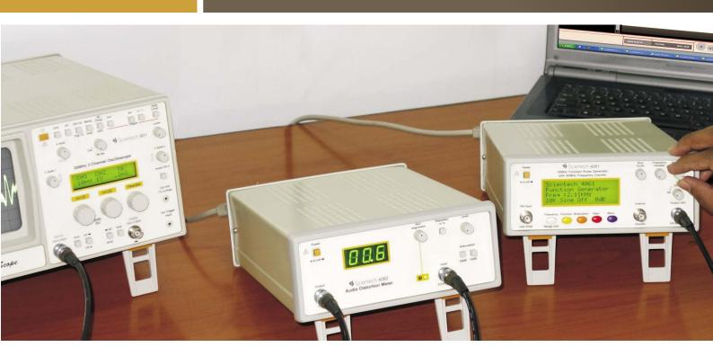
a minimum residual Distortion and Noise of 0.005%. It is best suited for measurement & testing of high quality Audio Systems. Scientech 4092 comes with a calibrated monitor output for Spectral Analysis and Visual inspection of input signal after filtering out the fundamental. Scientech 4092 has a resolution of 0.1%, Automatic frequency range selectors, and Automatic frequency nulling with 15% capture range. Scientech 4092 is a must for all Distortion
