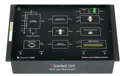
**Scientech 2309 Water Level Measurement** is designed to learn concept of Water Level Measurement. It helps students & industry professionals to understand operation of level sensors in detail. Built-in On/Off Controller is also provided with audio & visual indicators. It also has a PC interface through USB for more interactive understanding of Water Level Measurement. User can also take a direct printout if desired.
