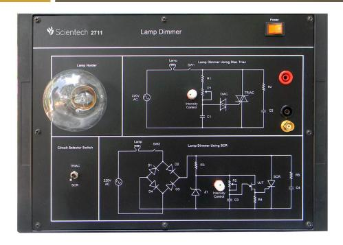
**Scientech 2711** is a comprehensive learning platform which is very useful for Students to understand the application of Thyristor in intensity control. Two firing methods are provided with this platform internal power attenuattor is included for observation of high voltage signals on the Oscilloscope. This platform is provided with internal AC/DC power supplies & exhaustive learning material.
